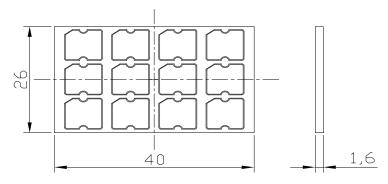
Unit: mm Tolerance:  $\pm 0.30$ mm
