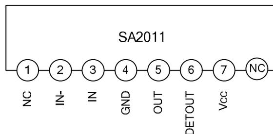
**Note:** When the seal is looked in positive direction, the left pin on the bottom is the first pin (Pin 1).
