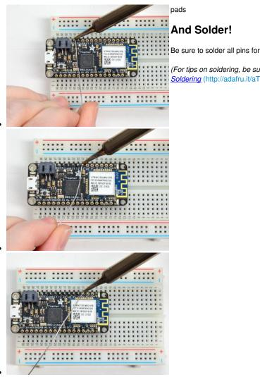
Be sure to solder all pins for reliable electrical contact.
