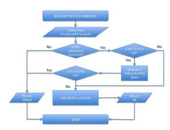
Note: The TX FIFO full check will happen for each GATT transaction (of up to 20 bytes of data each), so large data transfers may have multiple 200ms wait states.
