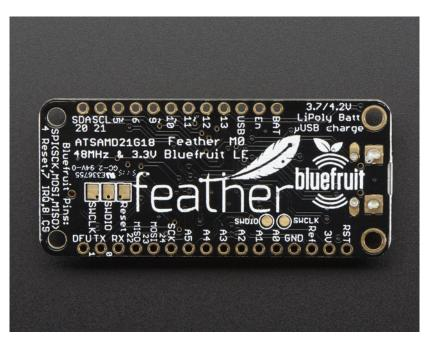
The Feather MO Bluefruit uses the extra space left over to add our excellent Bluefruit BTLE module + two status indicator LEDs
