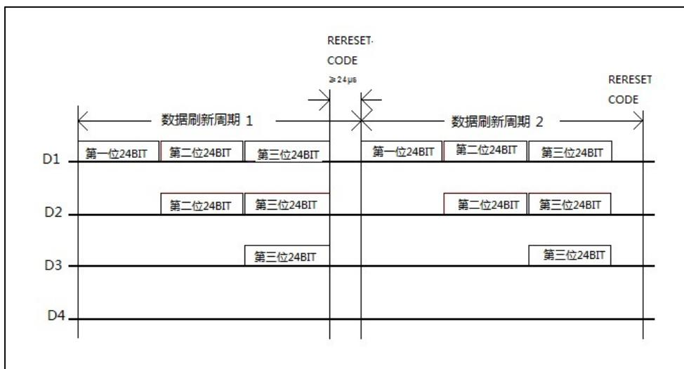
Note: the D1 for MCU send data, D2, D3, D4 for cascade circuit automatic plastic forwarding data.
